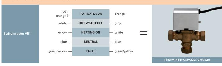
Switchmaster valve is not sprung return hence the extra wire (orange) to move the paddle into the hot water ON position. Insert link on junction box between red and orange of old valve and wire orange to orange.
