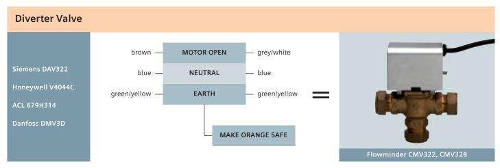
To replace a diverter valve with a mid-position valve, replace old brown wire with grey and white together and make the orange safe.
