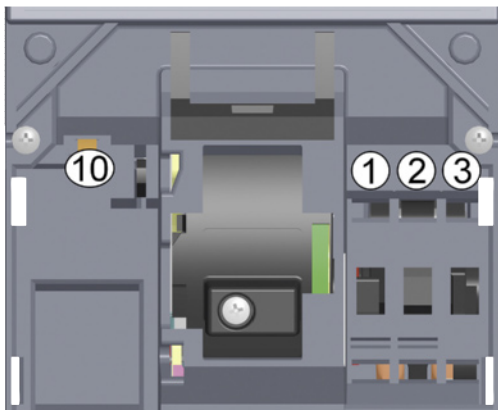
Location of accessory compartments 10 in 3VT2 circuit breakers
