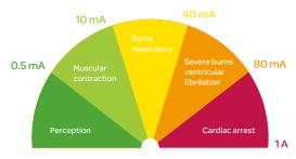
Research worldwide shows that the intensity of current flowing through the body determines the extent and severity of an electric shock.
