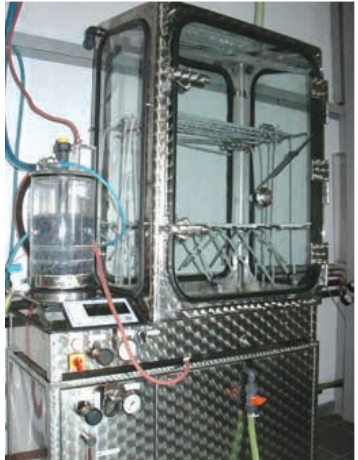
Environmental ageing chamber for ammonia atmosphere ageing
