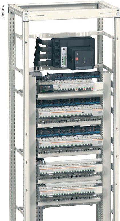
Compact NSX400 with motor mechanism, supplying rows of Multi 9 devices via Powerclip insulated busbars.
