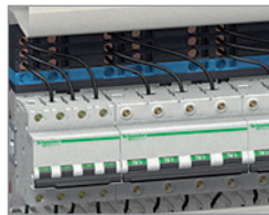
Linergy FM device feeder 80 A. The Linergy FM device feeder snaps easily onto the back of the rails. All types of modular devices can be mixed in the same row and phase balancing is simple. It's easy to change or add devices.
