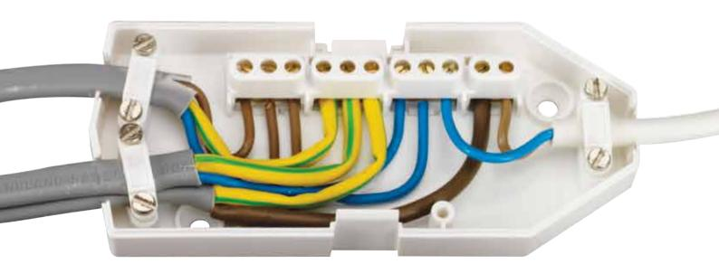
Regulation 526.2 is complied with where the method of connection shall take account of the number and shape of wires forming the conductor. In this junction box solid conductors and flexible conductors can be terminated separately by means of the unique three plate style terminal arrangement.
