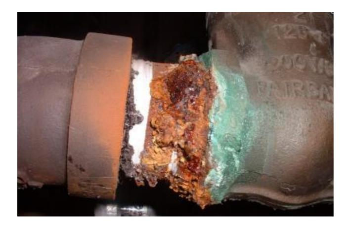
Galvanic or bimetallic corrosion occurs when two dissimilar metals are immersed in a conductive solution and are electrically connected. One metal (the cathode) is protected, whilst the other (the anode) is corroded. The rate of attack on the anode is accelerated, compared to the rate when the metal is uncoupled.
