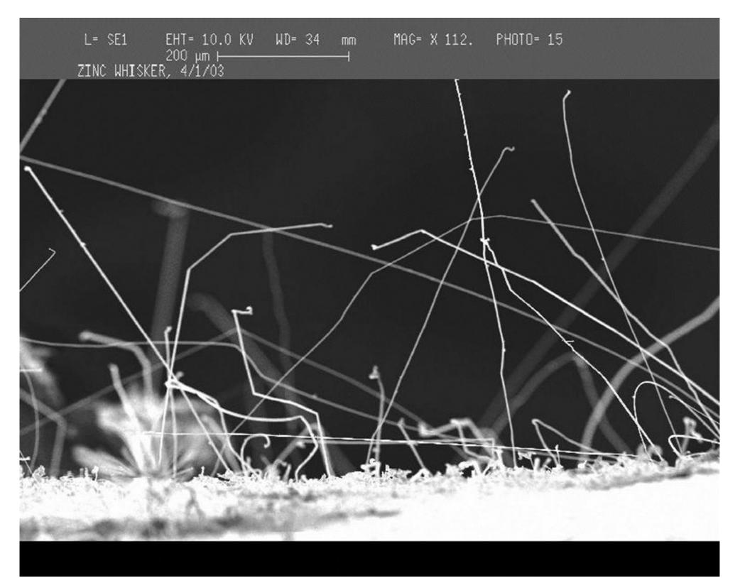
A naturally occurring crystalline metallurgical phenomenon where metal grows fine filiform hairs. Although primarily found on galvanised (electroplated) surfaces they can also occur on alloys.
