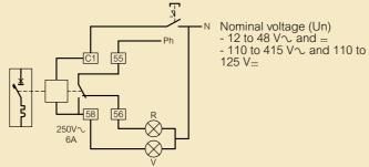
Equipped with a signalling contact which indicates tripping of the shunt trip and automatically breaks the coil.
