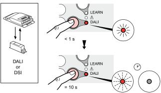
DALI Ballast: total lighting of all loads, then gradual dimming and switching off of the loads in a random order.
