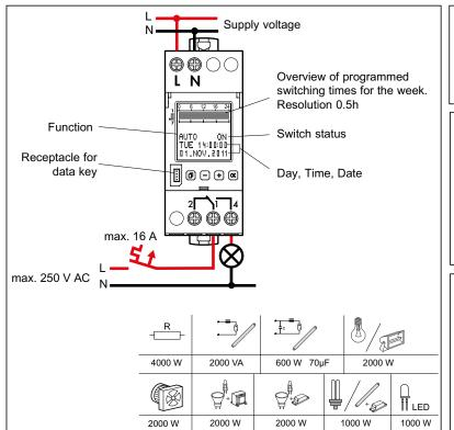
Operating principle: Typ 1.B. S. T. IEC/EN 60730-1, IEC/EN 60730-2-7 Operation in a normal environment
