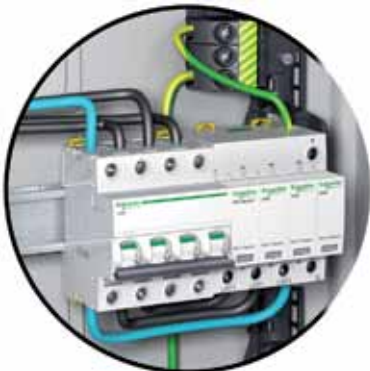
Surge arrester iPRD 3P+N + iC60N 3P+N for TT or TN-S (Incoming through the top without comb busbar)
