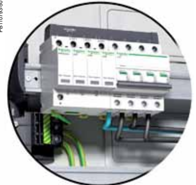
Surge arrester iPRD 3P+N + iC60N 3P+N for TT or TN-S (Incoming through the bottom with comb busbar)
